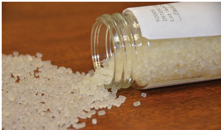
Above: The biocidal active ingredient is encapsulated in the carrier resin in Valtris's Intercede DBF-10-SVC pellets
