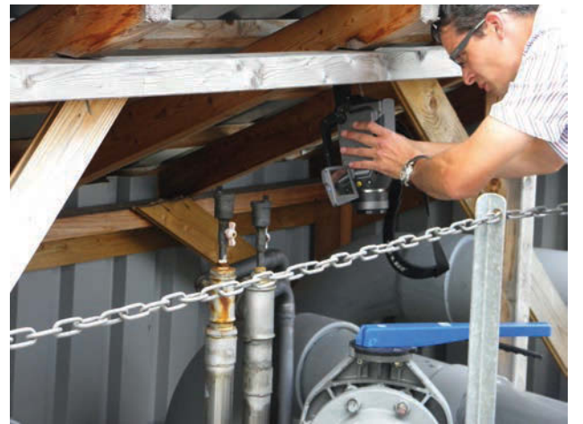
Engineer Ibeling van Lessen looking for gas leaks, which is possible from a safe distance and unusual angles using the FLIR GF320.
