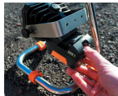
Fig 2.0. A lithium ion I.S. battery pack being hot swapped
